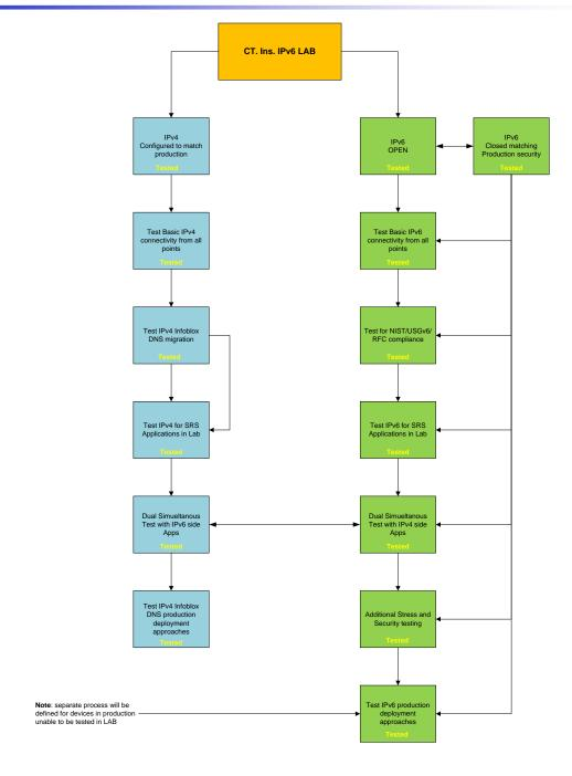
Figure 19 – IPv6 Lab Testing Flowchart
